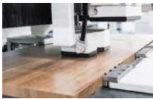
Panel hold-down device with rubber feet guarantees accurate processing
