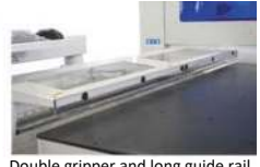
Double gripper and long guide rail
