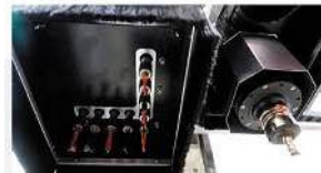
HSD Spindle: 9.6kw + Italian drill group(5+4 vertical drills)
